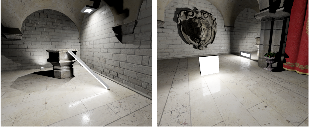
Fig. 12. Real-time rendering of photometric lights with our method and specular shading extension. The shadows are rendered point-based using cube shadow maps.
