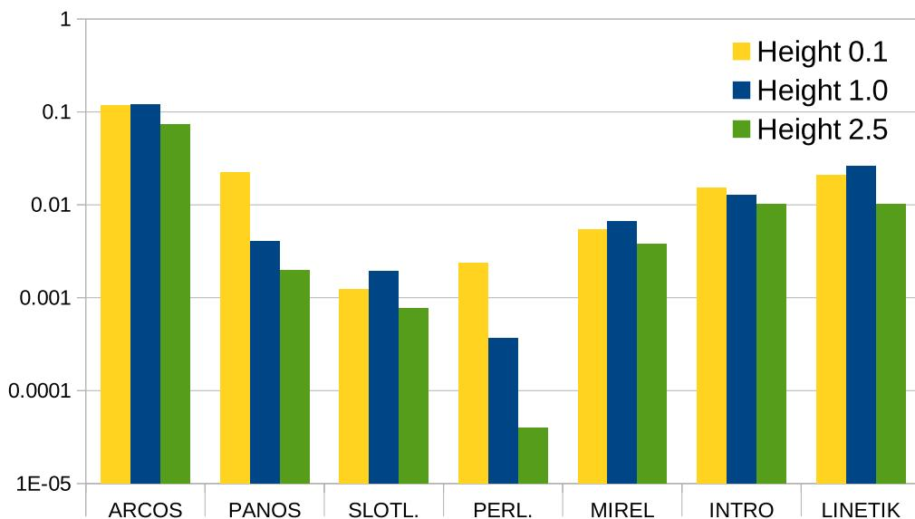
Figure 1: NRMS error of combined images with all orientations at different heights.
